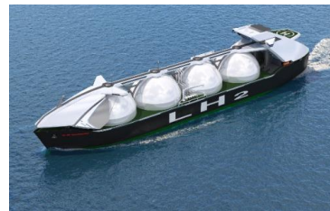
The 160,000 m 3 liquefied hydrogen carrier
